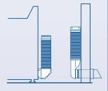
2 Extend vent toward top of dryer, then push dryer to wall.
