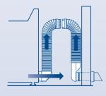
From over the top, snap vent together. Use extra clamps or extension collar to offset if needed.
